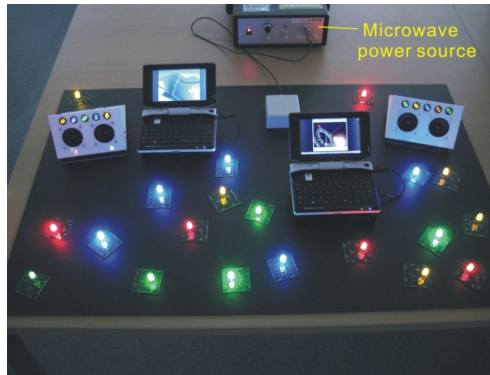
Fig. 12. Power supply via the communication sheet to small devices including speakers, LED lights, monitors, etc.
