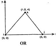
The nodal co-ordinates for an axisymmetric triangular element are given below. 7.
