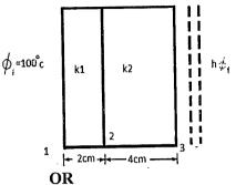
Find the temperature distribution in a square region with uniform energy generation as shown [10M] 9. in fig. Assume that there is no temperature variation in z-direction. Take k=30W/cm°c, length = 10cm,  $T_{\infty} = 50$ °C, q = 100W/cm<sup>3</sup>
