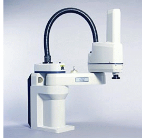
Figure 2.15 Articulated arm robots working in the cylindrical coordinate system: with the horizontal axis and vertical axis
