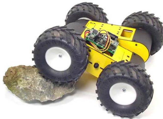
Figure 2.35 Example of a vehicle for moving on an uneven surface
