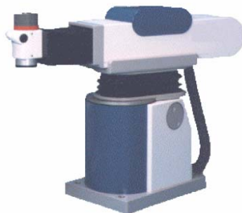
Figure 2.13. Manipulator in the cylindrical coordinate system: a working envelope for vertical axis robot, b working envelope for horizontal axis robot, examples of Versatran, Seiko RT3300 and Fanuc M300 robots
