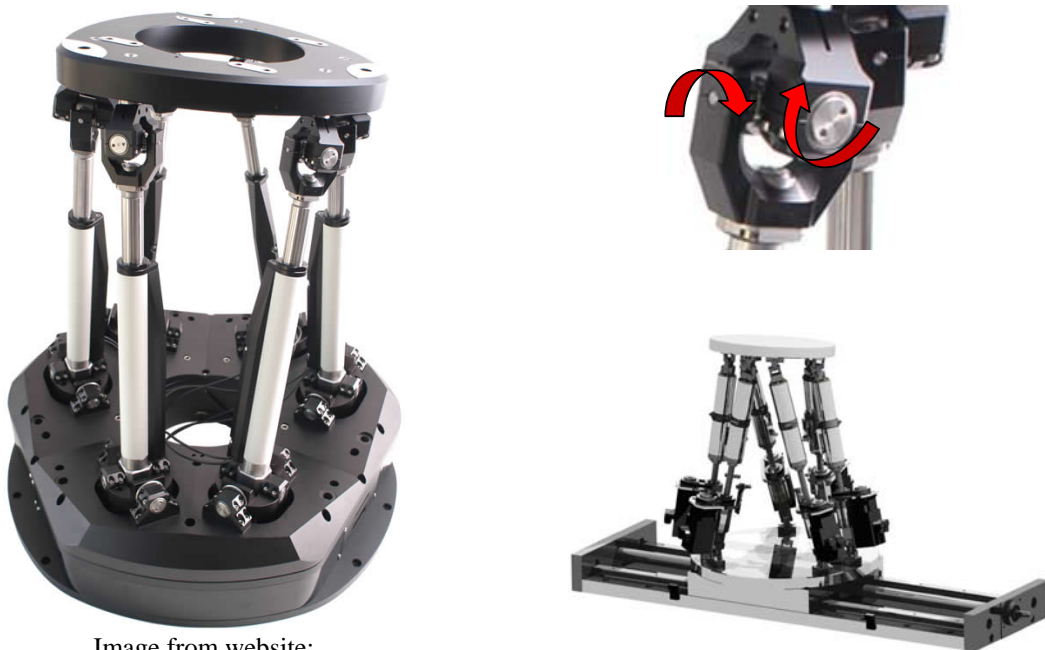
Figure 2.24 Six-leg hexapod manipulator and its constructional components
