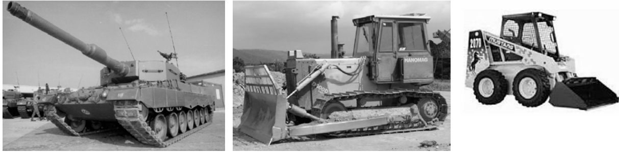
Figure 2.36 Machines using a crawling driving mechanism and brakes for turning (Photos of Uwe Berg from Internet)
