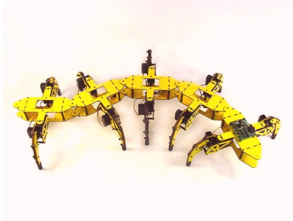
Figure 2.40 Ten-leg robot that moves by the turning pairs of legs
