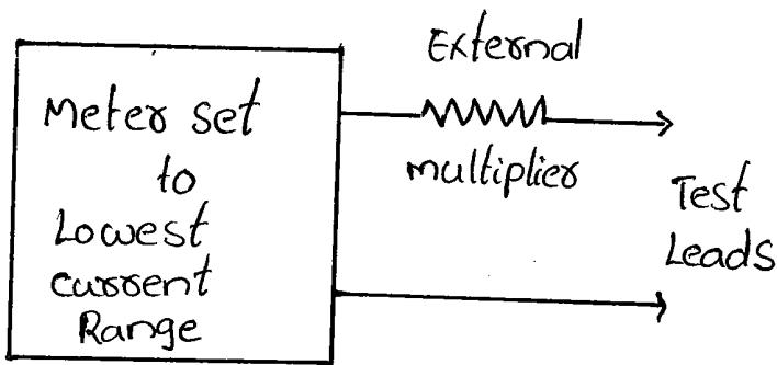
However great care must be used not to exceed the voltage drop required for full scale deflection of the basic movement.
