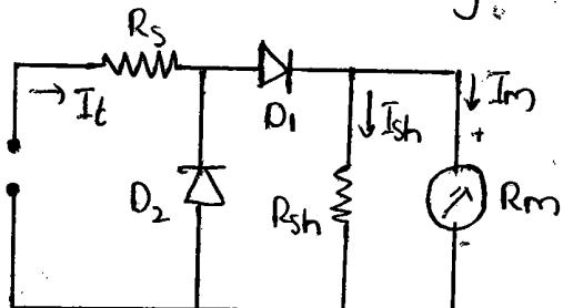
Diode  $D_1$  conducts during the positive half of the input cycle & causes the meter to deflect according to the average value of this half cycle. The meter movement is shunted by a resistor,  $R_{sh}$ , in order to draw more current through the diode  $D_1$  & move the operating point into the linear portion of the characteristic curve. In the negative half cycle, diode  $D_2$  conducts & the current through the measuring circuit, which is in an opposite direction, bypasses the meter movement.
