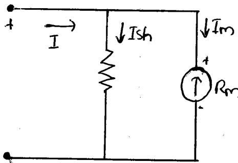
The resistance of shunt can be calculated using conventional circuit analysis.
