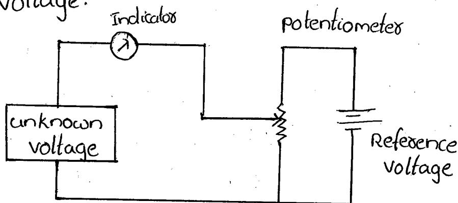
Figure shows a basic circuit of a differential voltmeter based on the potentiometric method; hence it is sometimes also called a potentiometric voltmeter. In this method, the potentiometer is varied until the voltage across it equals the unknown voltage, which is
