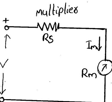
To measure the potential difference between two points in a dc circuit, a dc voltmeter is always connected across them with the proper polarity.
