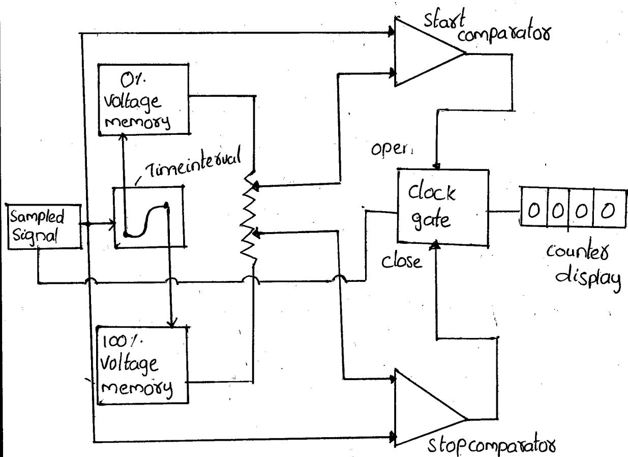
The input signal is first sampled using sampling circuit. The sampled signal is given as one output to each start & stop comparators. When input is sampled, the Sampling circuit advances the sampling position by a fixed amount. This process is called strobing. The selected sweep time per cm control & number of samples taken per cm decide the equivalent time between two samples.
