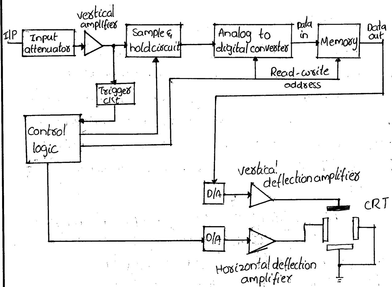
As done in all the oscilloscopes ; the input signal is applied to the amplifiers & attenuators section . The oscilloscope uses same type of amplifiers & attenuators circuit as used in the conventional oscilloscopes. The attenuated signal is then applied to the vertical amplifiers
