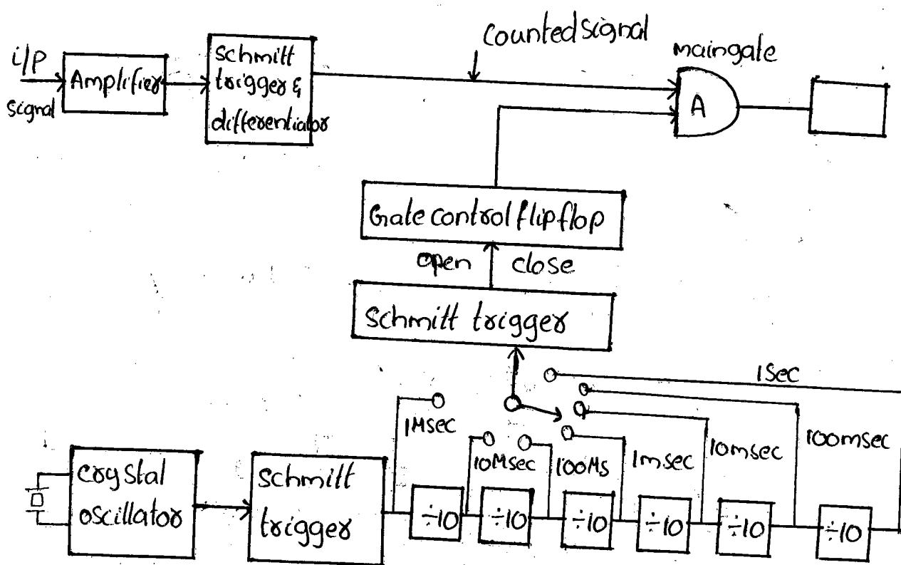
When the output of the And gate is high, it is counted as 1, irrespective of the shape. The wave shape is not important for counting.
