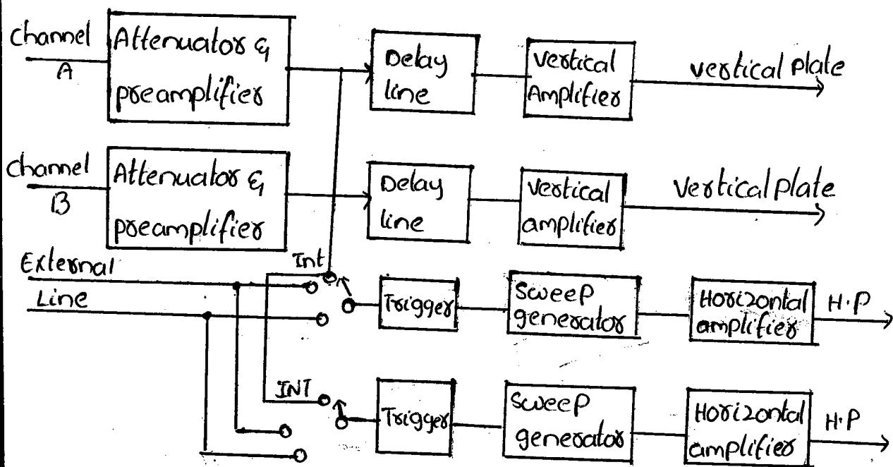
The dual beam oscilloscope has two separate electron beams, therefore two completely separate vertical channel. The two channels may have a common time base system or they may have independent time base circuits as shown in figure. An independent time base allows different sweep rates for two channels but increases the size & weight of the oscilloscope.
