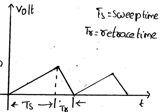
damp voltage & the fact that the positive voltage attracts the negative electrons. During the retrace time or fly back time  $t_0$ , the beam returns quickly to the left side of the screen. The control grid is generally "gated off" which blanks out the beam during retrace time & prevents an undesirable retrace pattern from appearing on the screen.
