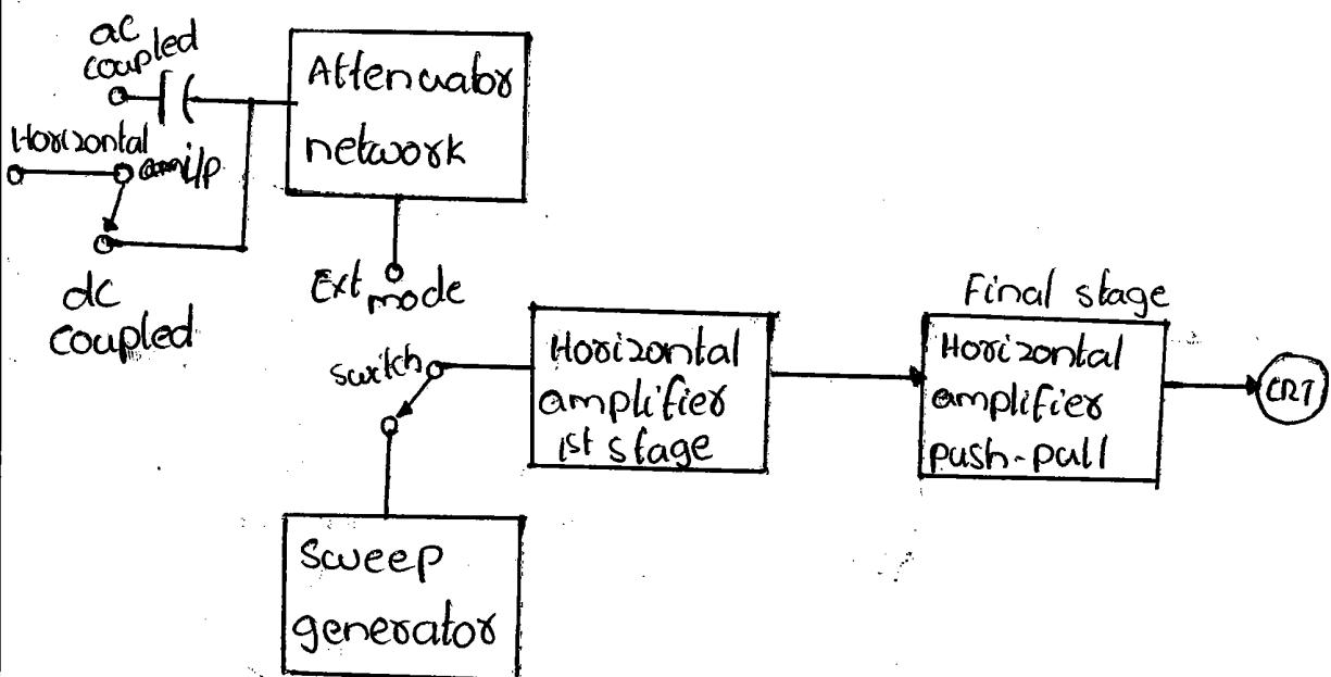
The attenuator network given in the figure reduces, by voltage division, the amplitude of the horizontal input signal to a level equal to the sensitivity of the horizontal amplifier.
