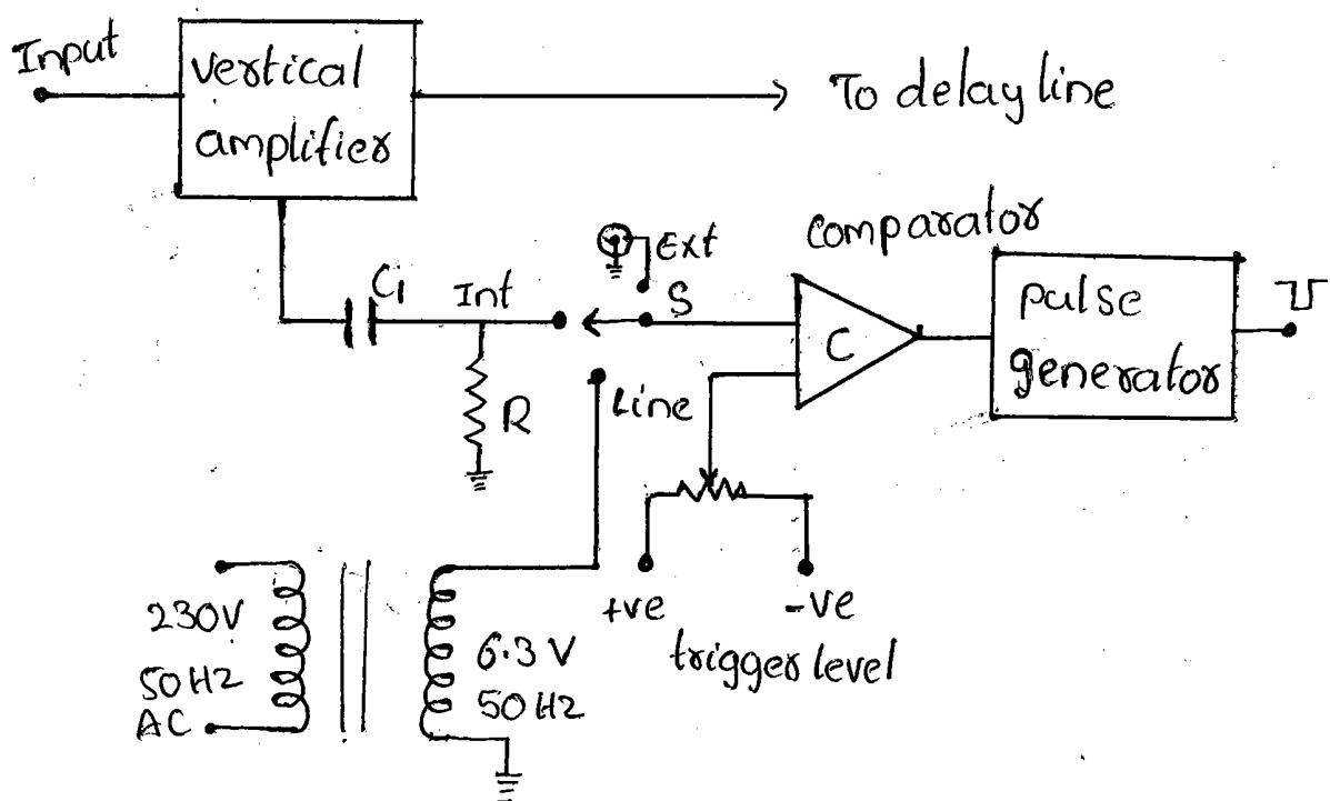
The trigger section is a 3-position switch. Internal-External-Line. The trigger input signal is applied to a voltage comparator whose reference level is set by the Trigger Level control on the CRO front panel.
