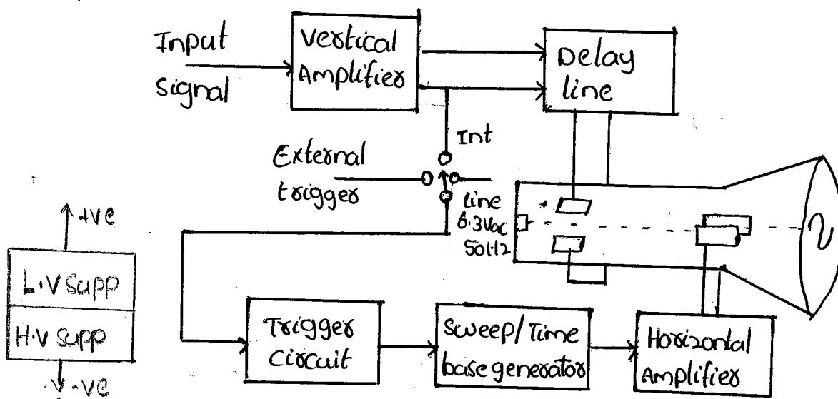
The cathode ray oscilloscope is a very useful, general purpose electronic instrument for testing & developing electronic circuits, systems & instruments.
