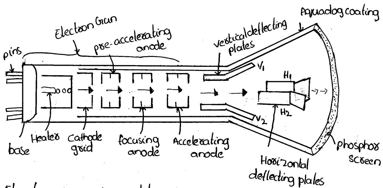
**Electron Gun Assembly:** The electron gun emits electrons & forms them into a beam. This beam is focused on to screen to cause a luminous spot on the screen.
