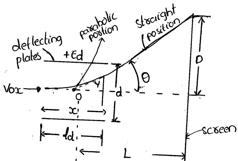
There are two parallel plates with a potential applied between. These plates produce a uniform electrostatic field in the  $y$  direction. Thus any electron entering the field will experience a force in the  $y$  direction & will be accelerated in that direction.
