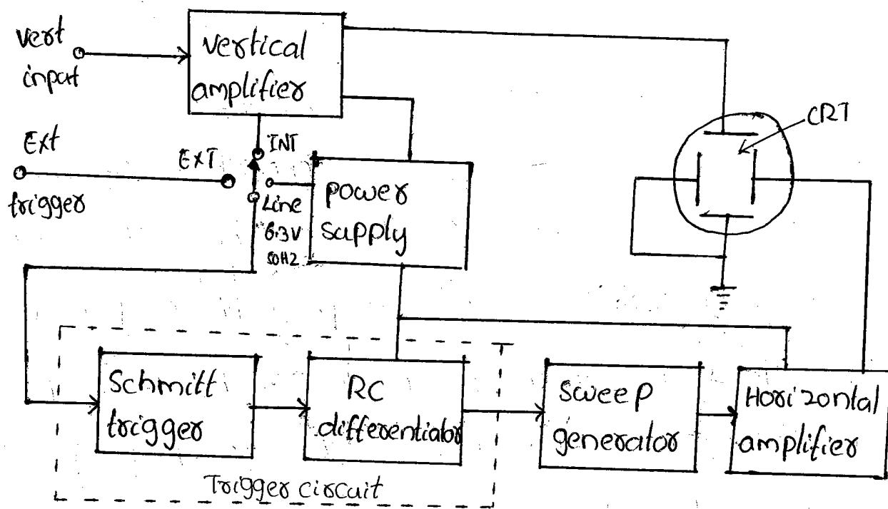
The trigger circuit may receive an input from one of three sources depending on the setting of the trigger selector switch. The input signal may come from an external source when the trigger selector switch is set to EXT, from a low amplitude
