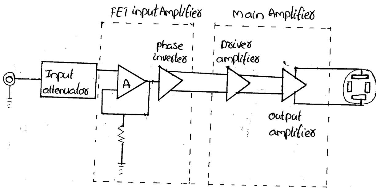
The vertical amplifier consists of several stages with fixed overall sensitivity or gain expressed in V/div. The advantage of fixed gain is that the amplifiers can be more easily designed to meet the requirements of
